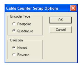
When the type has been set-up, click the OK button. The cable counter should normally be calibrated after this.
